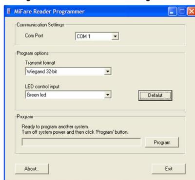
3. In Communication Settings, set **Com Port** to the port that the MD-08B is connected to.
