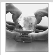
To open the receiver, expand the two sides of the box and lift up the cover.
