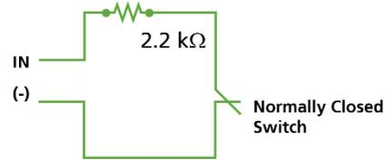
Normally Closed Supervised inputs with a single resistor must be connected with a 2.2K resistor in series to the input switch contacts.
