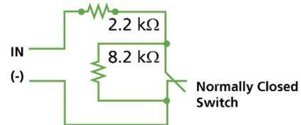
Normally Closed Supervised inputs with two resistors must be connected with an 8.2 K resistor in parallel and a 2.2 K resistor in series to the input switch contacts.
