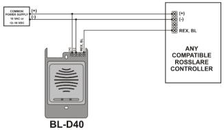
It is recommended that 22 Gage wire be used between the BL-D40 and the controller.
