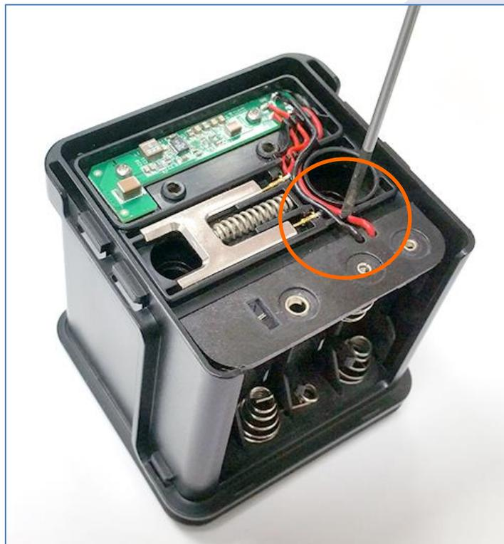
Place the top cover back and use the cross-head screwdriver to screw back the two screws.
