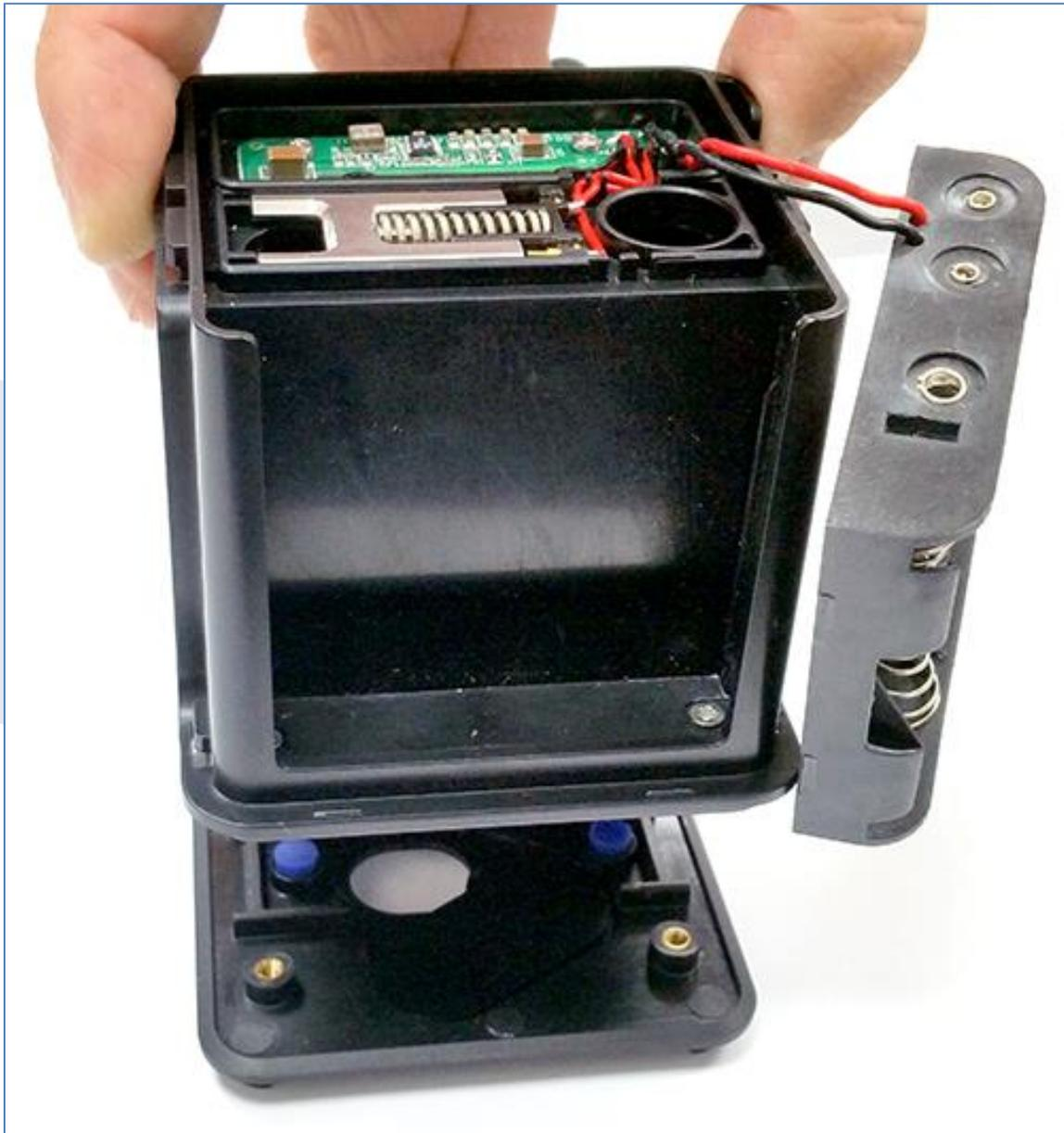
Use the cross-head screwdriver to screw back the two screws underneath the battery holder.
