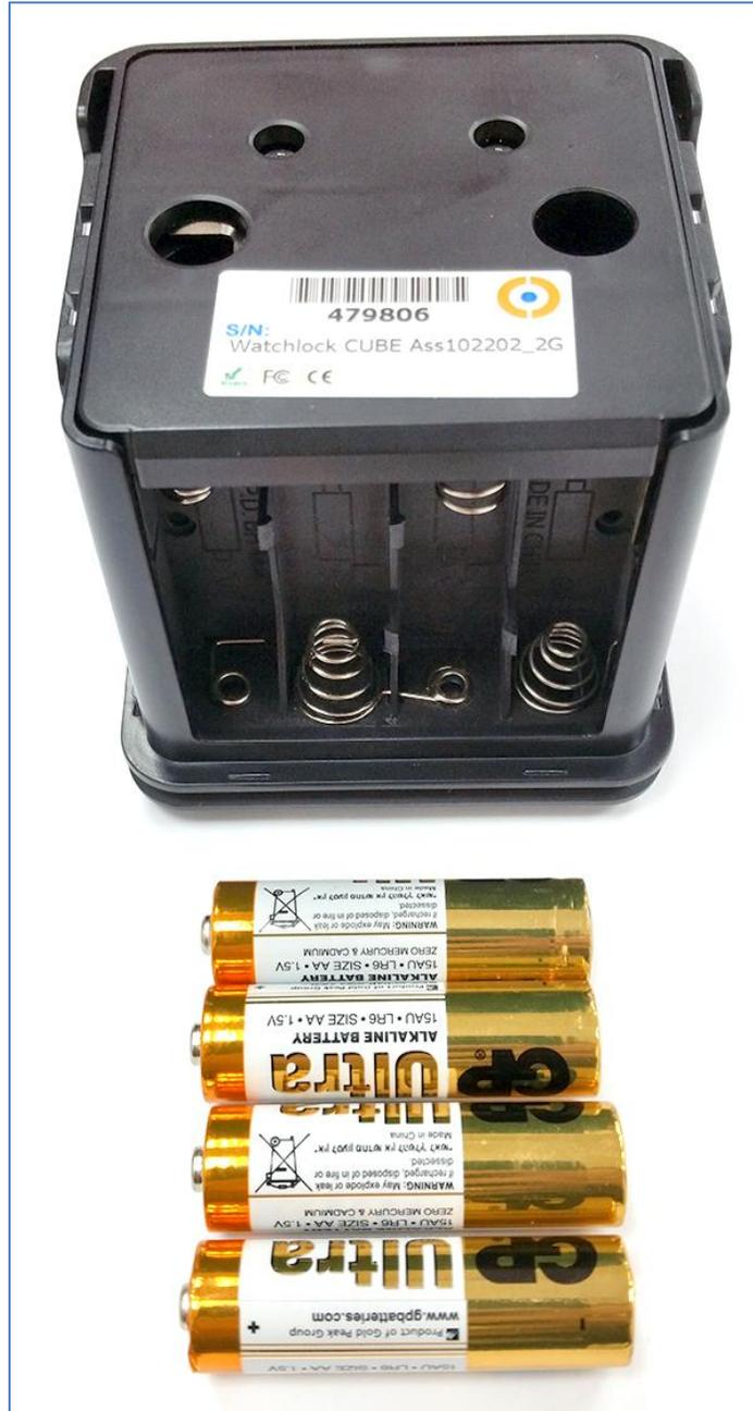
Carefully insert each battery according to the polarity markings on the battery holder, ensuring that the + (plus) and - (minus) terminals are aligned correctly.
