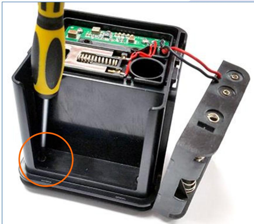
Carefully slide the battery holder back in its place.
