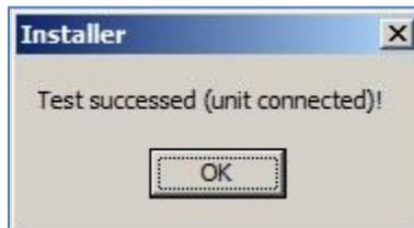
If at the end of the TCP Test you do not receive a successful message, check your APN settings (Watchlock Parameters > Network). Contact your cellular provider and make sure the SIM card is open for GPRS. Verify that your SIM card is not protected by a PIN code. If necessary, use a mobile phone to cancel the PIN code.
