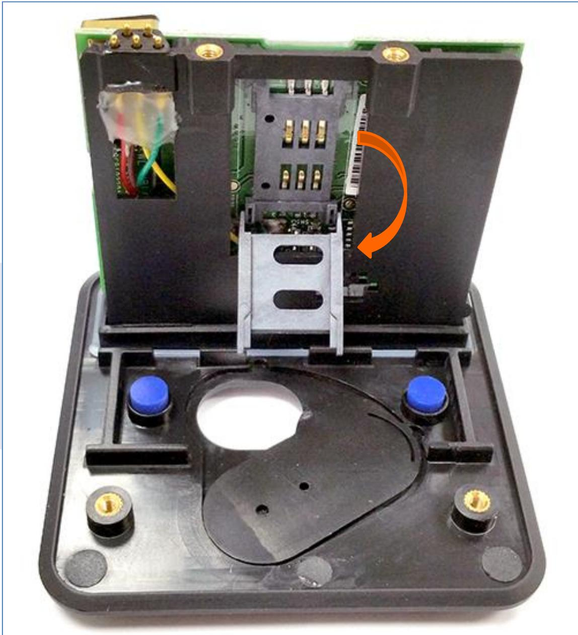
Insert the SIM card into the SIM card slot with its gold contacts facing you and its cut-off corner facing out the SIM card slot, as shown in the following image.
