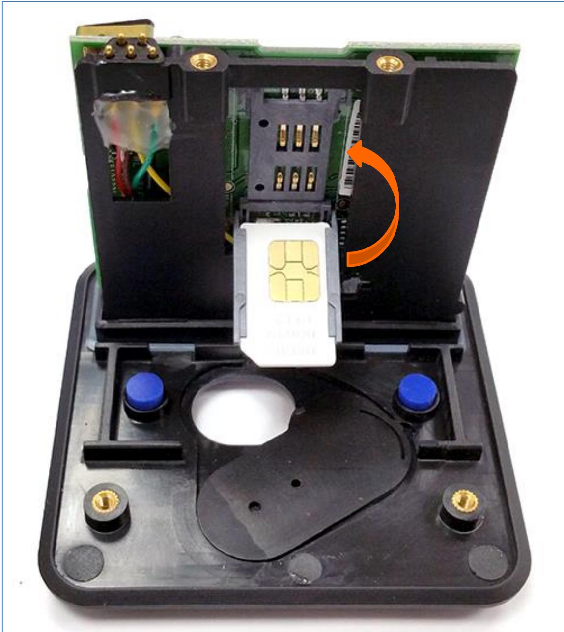
Put the SIM card holder back into vertical position. Gently press and push the SIM card holder forward to snap it back into place.
