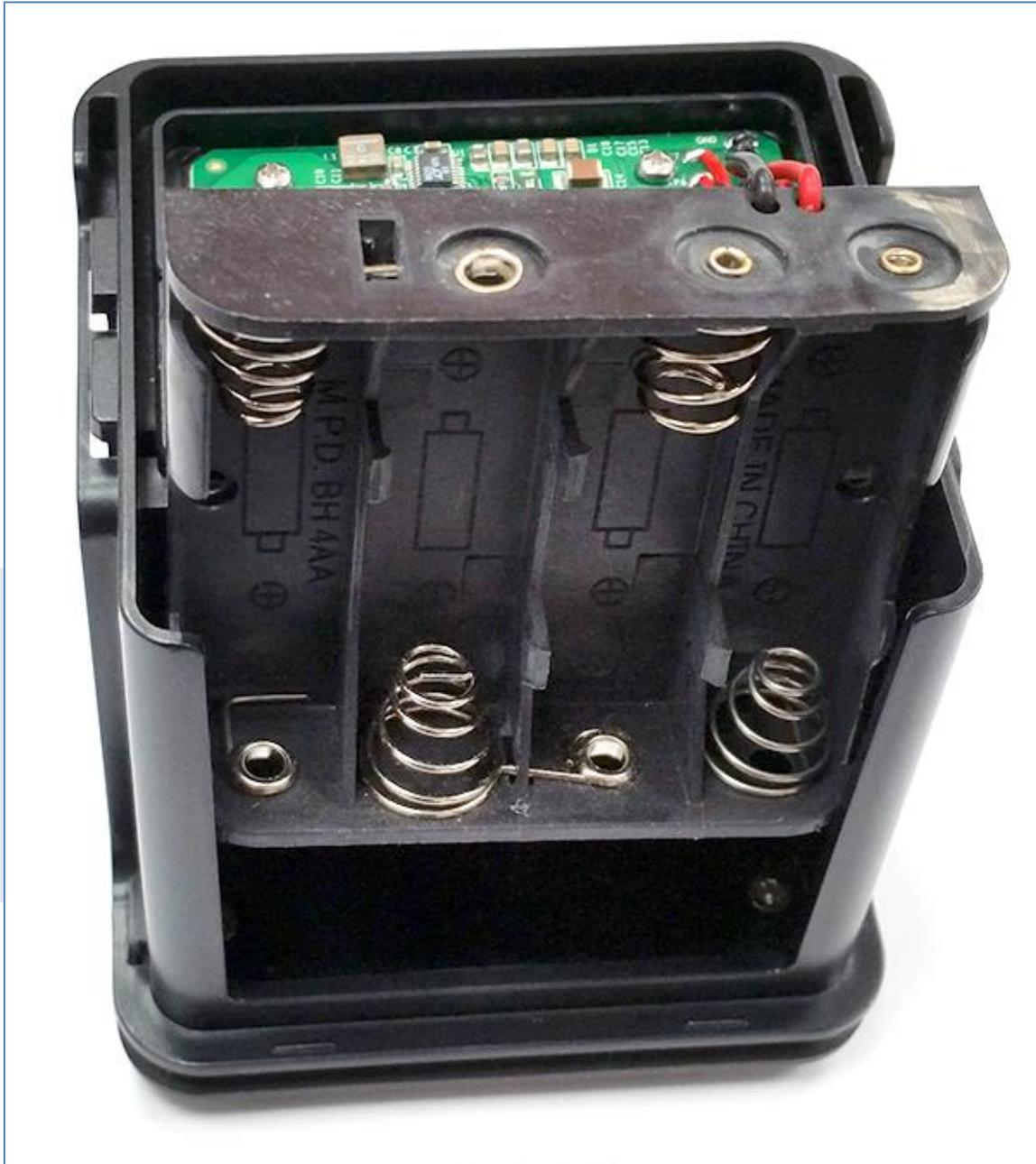
Place the wires back in the track. If necessary, use a small, flat screwdriver to carefully fixate the wires.
