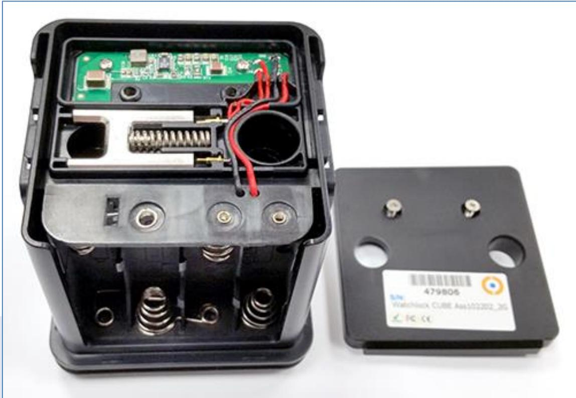
Carefully pull and slide out the battery holder.
