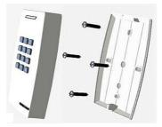
Figure 1: Removing Back Cover
