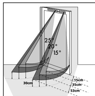
Overview of the sensing fields as a function of module placement angles.
