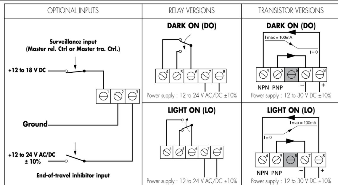
**REMARK :** If an inductive load is connected (operator relay), put a protective diode.
