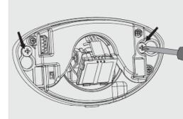
3. Connect power cable to sensor's terminal
